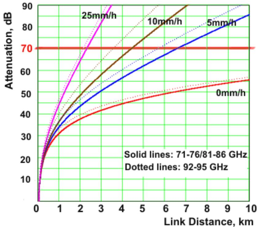
Fig.1 Distance versus rain graph for FCC E-band. The transceiver sensitivity limit for gigabit links line is 70 dB
